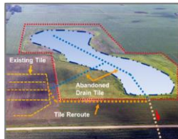
Figure 3. Drainage Tile Rerouted Around a Restored Wetland
